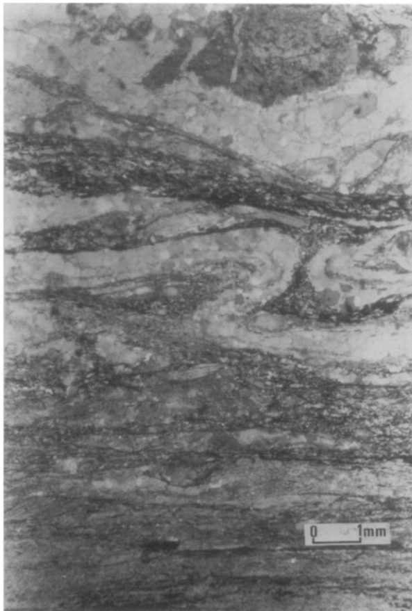
Fig. 7. Asymmetric microfold deforming the S and C surfaces compatible with the proposed dextral simple shear. Scale bar is 1 mm.
